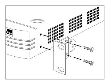
**Figure 7** Fitting a bracket for rack mounting
